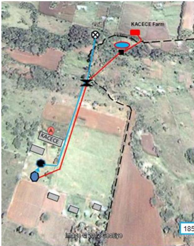
⊗ Water is collected from the springs source. Gravity feeds water down to the lower area
